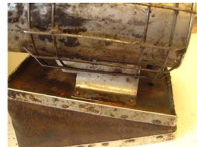
14. Replace the grate being careful to place a leg on either side of the inlet tube. Replace the bellows and tighten the 4 nuts. Putting a little oil on the threads makes the job easier next time.
