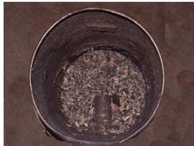
8. You may find debris and/or soot in the can under the grate. Scrape this and dump it out.
