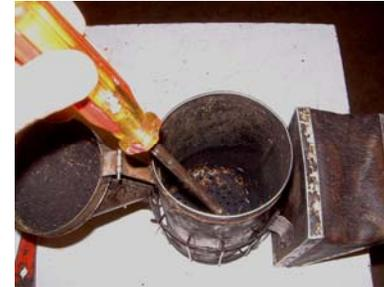
4. You do not have to get it perfect but remove the majority of the soot and carbon. Removing the crud from the can makes it easier to get the grate out in the next step.
