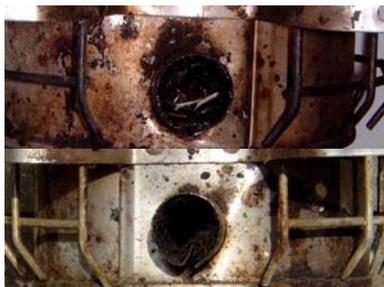
12. Sometimes the tube is completely plugged like the top one. It only takes a partial plug like the bottom one to make the smoker operate poorly.
