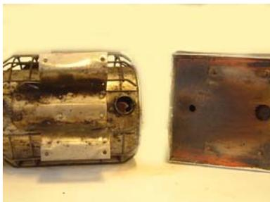
11. Separate the smoker from the bellows and clean the tube. Notice how clean this tube is.
