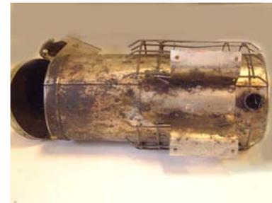
9. Often the air tube becomes plugged. I have tried many tools to clean this without removing the bellow. None are satisfactory, so remove the bellows.
