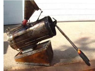
5. Remove the grate from the bottom of the smoker. I find it easiest to use a long nose pliers. Put one nose into each of 2 holes close to the edge and pull. You can also bend a wire or rod to fit in a hole near the edge and pull it up.
