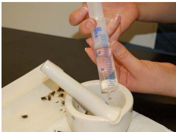
6. Add 0.1 ml of water for each bee (2.5ml water for 25 bee sample or 5ml for 50 bee sample).
