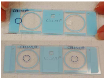
11. Slide the cover over until the viewing circle is about in center of the sample circle. Allow to rest for at least 63 seconds.
