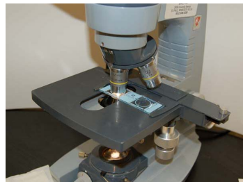
12. Place slide under microscope lens and find counting grid. Use low (100X) power until you find the grid and center it in your view. After you switch to high power (400X) use only fine focus adjustment so you don't accidentally break the glass counter.
