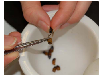
4. Remove abdomen (or guts) from 25 bees and put into mortar. For higher accuracy remove abdomen from 50 bees.
